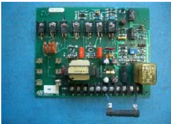
Figure 7: Top-view Photograph of the Constructed Converter.
