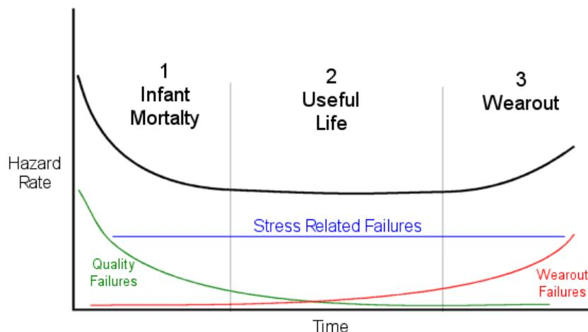
**Figure 1:** Bathtub Curve for a Mechanical or Electronic Components.
