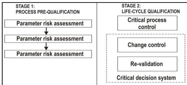
**Figure 5:** Two Stages of Process Validation.
