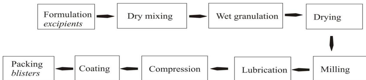
**Figure 3:** Stages in Tablet Paracetamol 500mg Manufacture.
