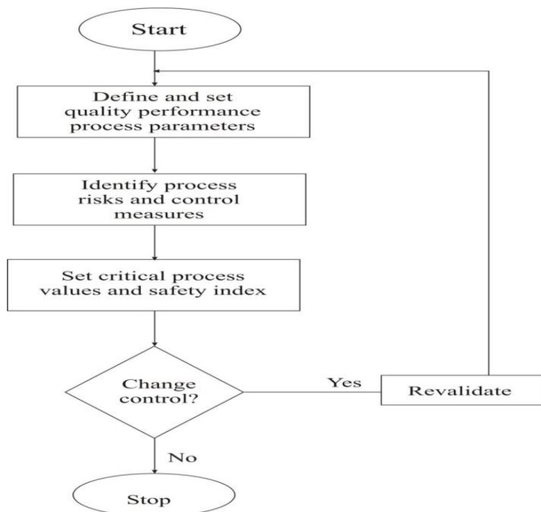
**Figure 2:** Flowchart of the Process Validation Process.
