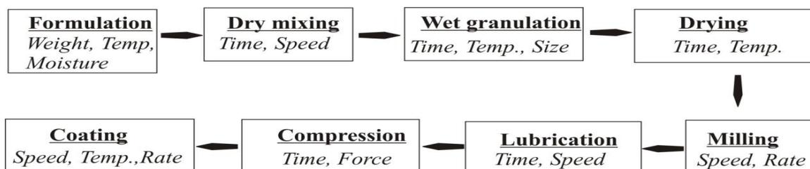
**Figure 4:** Tablet Paracetamol 500mg Production Stages showing CPVs.
