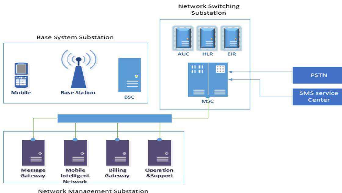
Figure 1: Subsystems in the GSM Standard.
