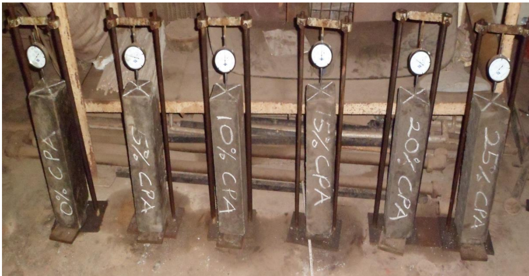
Figure 1: Experimental Set-up for Shrinkage of Cassava Peel Ash Concrete at Different Content of CPA.
