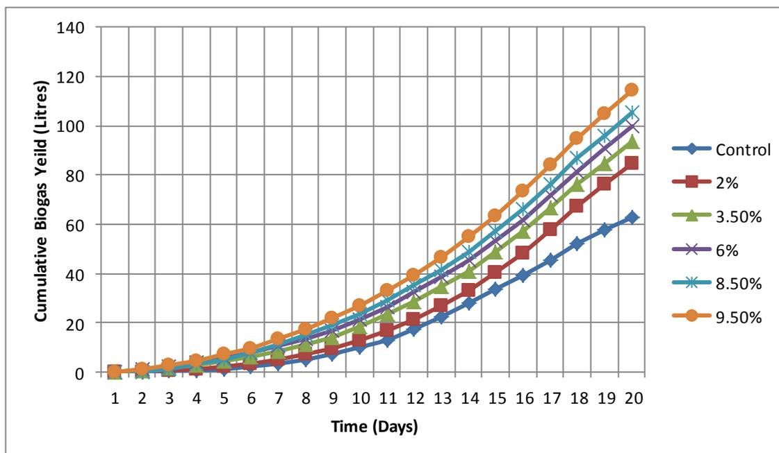
**Figure 4:** Cumulative Biogas yield (Liters) versus Time (Days).
