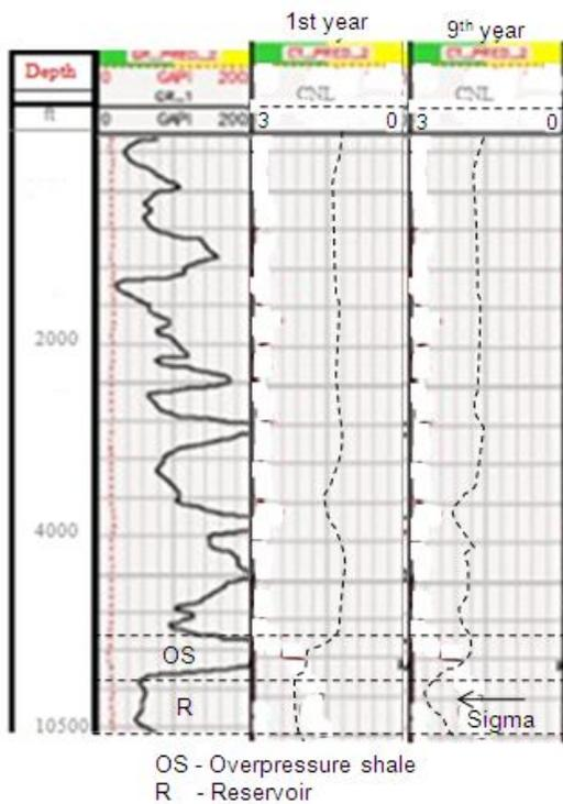
Figure 3: Pulsed Neutron Logs Run after Completion of Well A in Reservoir X.
