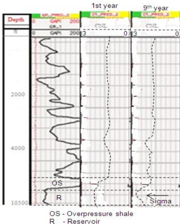
**Figure 5:** Pulsed Neutron Logs Run after Completion of Well C in Reservoir Z.
