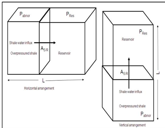
**Figure 1:** Diagrammatic Illustration of Shale Water Influx.
