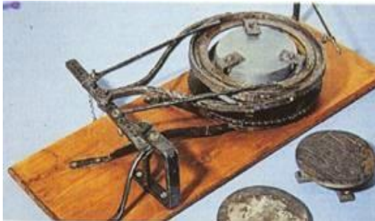
Figure 3: William Herschel's Polishing Machine (Source: Lord Rosse, 1841)
